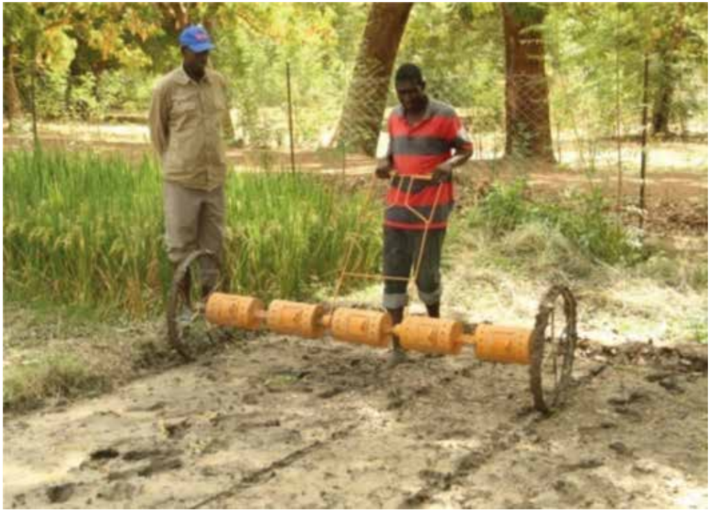
Figure 24: Demonstration of the newly adapted rice seeder at the Office du Niger.
