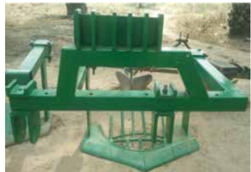
Figure 20: A mechanical cassava harvester developed by WAAPP NCoS on roots and tubers.
