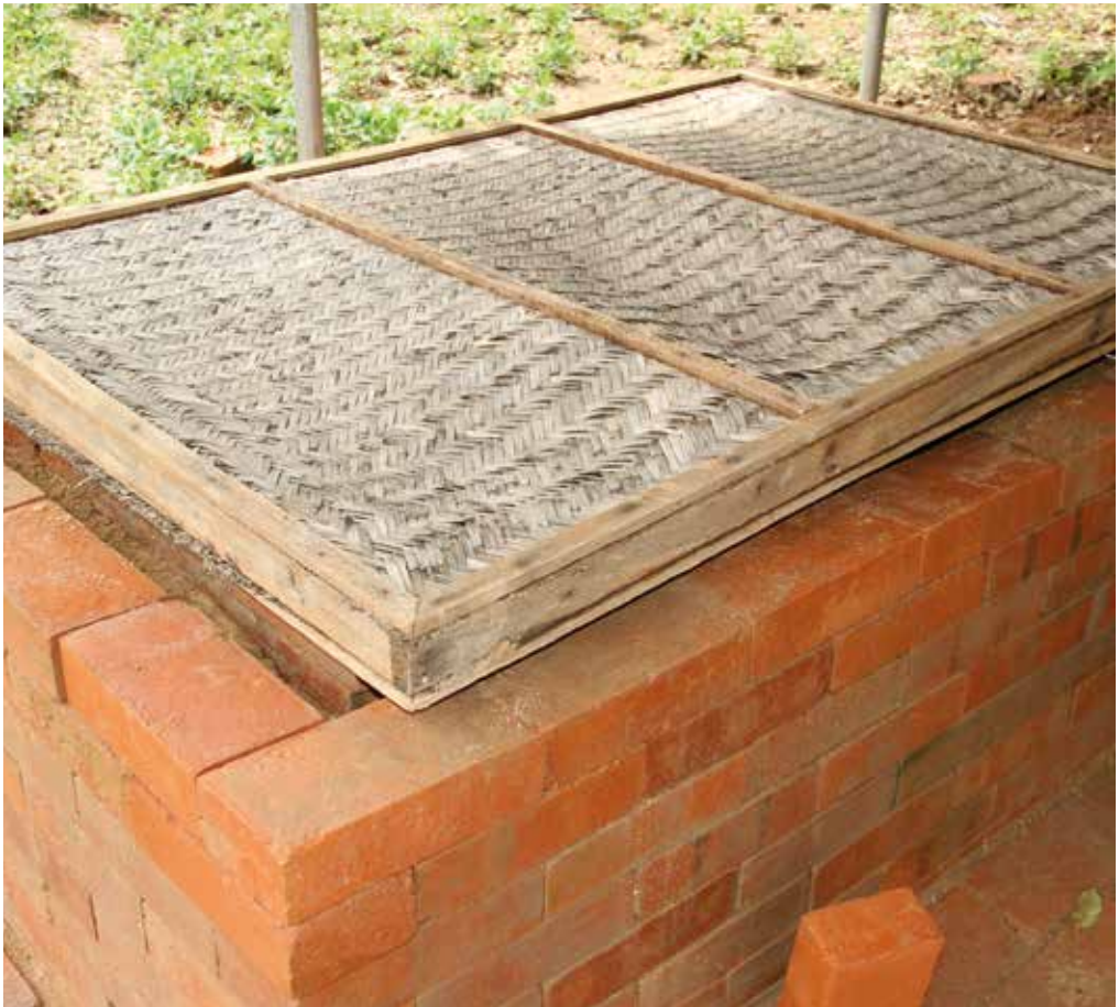
A Zero Energy Cooler Chamber
